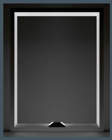
The structure of a façade can be emphasized by illuminating the window reveals. The result is the impressive highlighting of a building at night.
