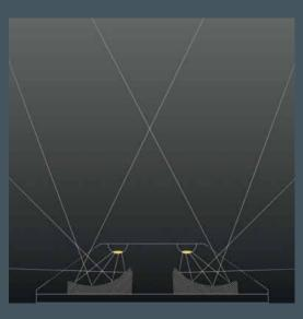
With the precise optical system the intensity of the light beam is adapted to varying distances from the luminaire to the window frame. Hence an optimal uniformity is achieved. Arclux RGBW creates the same effect with excellent colour mixing.
