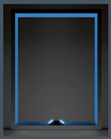
Arclux is a luminaire for the accent lighting of window reveals. The light from 2 LEDs is directed from the opposite sides of the luminaire, via specially developed reflectors, onto the widow reveal. The result is a uniform arc of light. A complete window reveal can be illuminated using just one luminaire.
